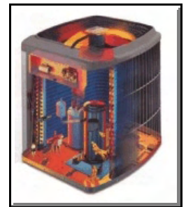
Cut away illustration of a typical heat pump.
