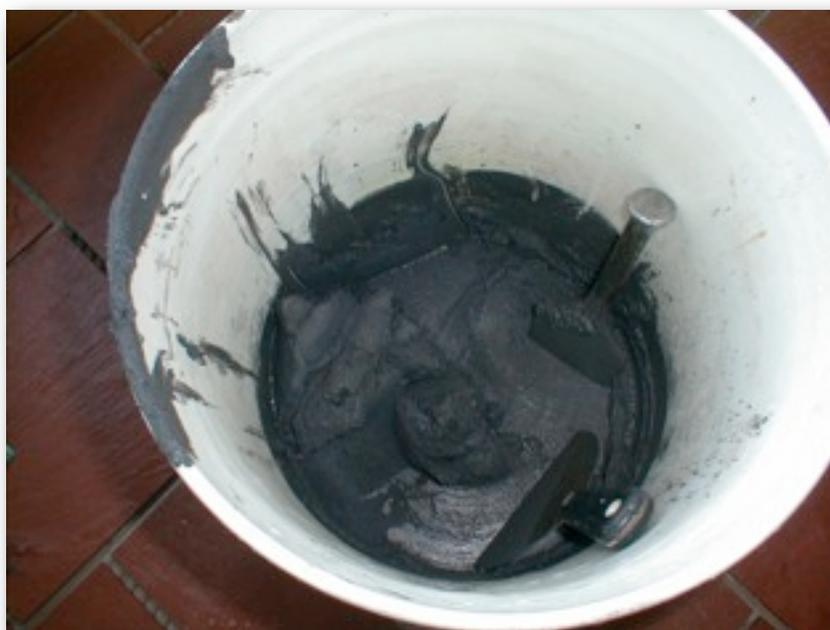
you added too much water. **Water is a vital ingredient when mixing grout, but too much water when mixing, finishing or cleaning the grout will ruin it.**
