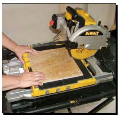
water flooding the edge of the blade. This water cools the blade thus increasing the cutting life of the blade. The water also eliminates dust. This allows you to use the saw indoors so long as you contain any water that may drip or spray away from the saw.
