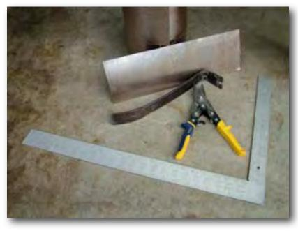
that there is no tape measure. I used the rulers that are embossed on the framing square. In this photo, you see the framing square, the tin snips, a pry bar and a flat piece of metal that's 5-inches tall by 24-inches wide. It was cut out of the coil of material that's standing upright in the top of the photo. The metal is tin-coated steel. It's actually 40-pound tin. This means it has 40 pounds of tin applied to 100 square feet of the metal. The more tin you have, the better.
