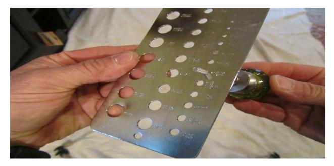
I first measure the knob screw to determine which size drill bit to use. Make sure to choose a hole that the screw loosely fits in without any friction or having to "screw it in."
