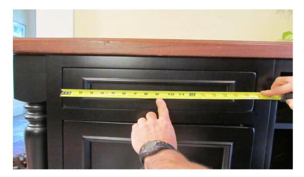
Determine the location of the hole(s) to be drilled from the side and bottom edge of doors, (for drawers measure from both sides and from bottom and top for centering) mark the hole positions on the masking tape.
