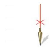
A plumb bob is a simple tool that delivers extreme accuracy when it's used properly. Using one of the simple laws of physics, a plumb bob is drawn to the center of the Earth. When it's not moving, the line supporting the cone-shaped machined brass is perfectly plumb.
